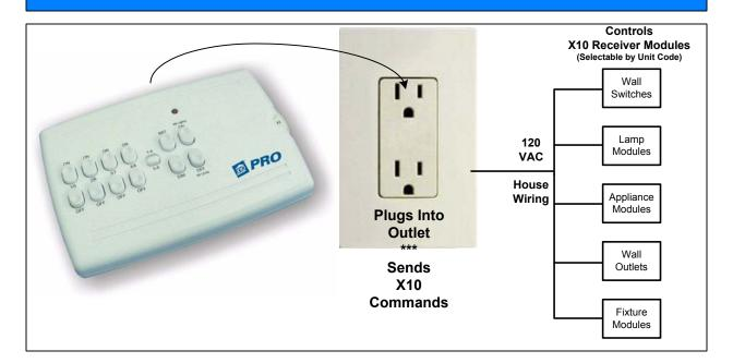
**Description:** The PMC01 Mini-Controller gives you manual control of up to eight X10 Receiver Modules of various formats. Just plug it in and you are in control! The PMC01 turns On/Off up to eight X10 lights and appliances connected to X10 Receiver Modules. The PMC01 has On/Off, Bright/Dim, All Lights On and All Units Off Command Buttons. The Selector Switch assigns the 4 On/Off Buttons to control the X10 Receiver Modules set to Unit Codes 1-4 or 5-8.
